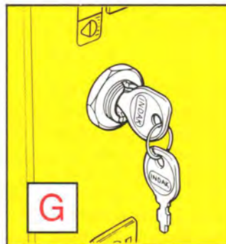
G IGNITION SWITCH
