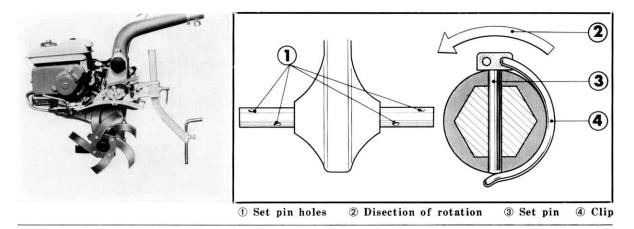
Depending on the width of crop and the soil condition, number of rotor blades will be changed from one to three blades on each side.
