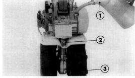
① Oil ② Oil level ③ Oil drain plug
