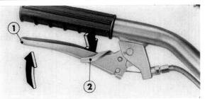
1 Clutch lever 2 Clutch lock lever
