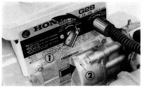
1) Engine switch (fuel cock) 2 Choke lever
