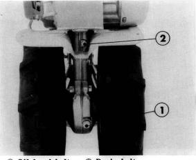
1 Oil level bolt 2 Drain bolt
