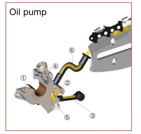
① Worm gear ② Oil pump piston ③ Suction line oil ④ Bearing Ball ⑤ Adjustment screw
