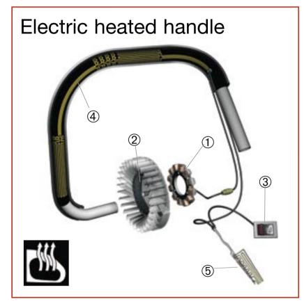
① Generator coil ② Flywheel with magnets③ Switch for handle heating ④ Heating foil in tubular handle ⑤ Heating foil in rear handle
