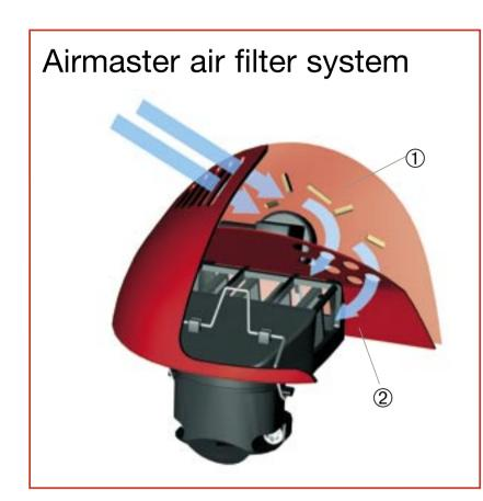
The maintenance friendly airfilter system retains the coarse particles in chamber ① and only the very fine particles access the airfilter chamber
