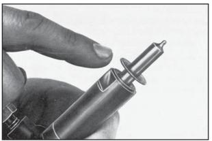
Adjustment is effected by inserting copper washers between the injector and injector supporting faces on the heads (fig. 76). Washer thickness 1 mm (RD210-211) and 0.5 mm (RD270-278).
