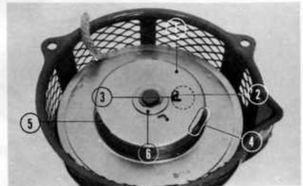
Fig. 1-8 ① Friction plate ④ Cutouts ② Set spring ⑤ Starter ratchets ③ Alignment ⑥ Washer B
