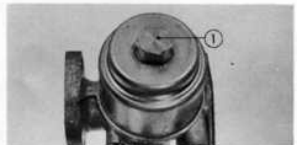
Fig. 4-10 ① Special bolt
