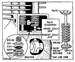
valve cover plate, oil spray shield, and breather valve. The correct valve clearances are as follows when the engine is cold:
