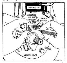
b. Turn crankshaft by hand to see if contact points open and close properly. Points must be clean and line up squarely to make good contact. Do not file points - use fine sandpaper or fine grit hone to clean points. e. Adjust gap to .020" by loosening the ad-
