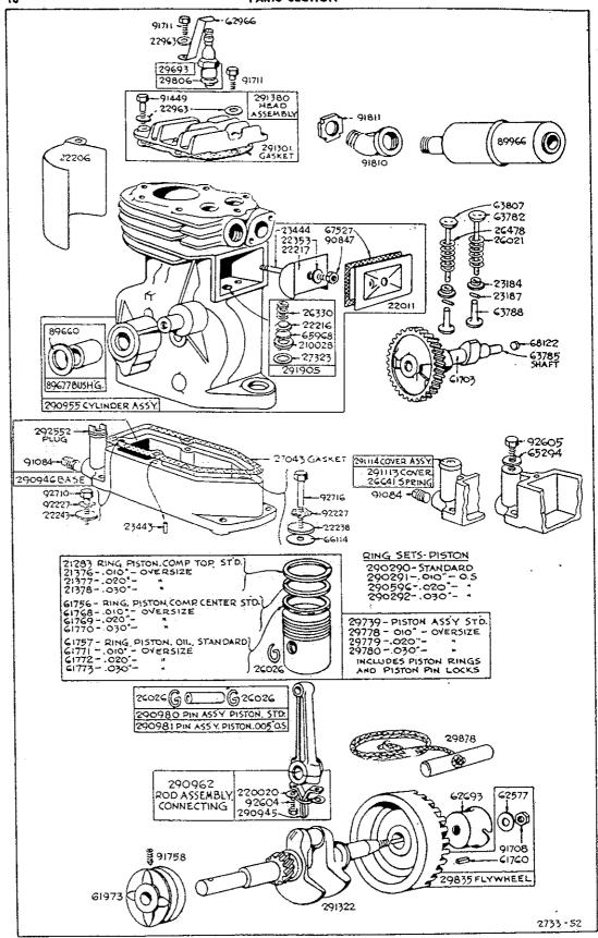
CYLINDER, PISTON, CONNECTING ROD, CRANKSHAFT AND FLYWHEEL PARTS — PLATE No. 20
