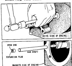
Be sure not to get burrs on the end of the shaft. After the shaft has been removed, check shaft for wear. If worn more than .001", replace with a new shaft.
