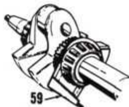
Fig. T28 - Oil slinger (59) on Models VH80 and VH100 must be installed on crankshaft as shown.
