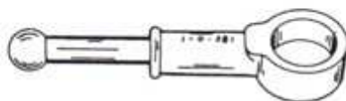
Fig. T27 - Install late type oil pump so large flat surface on drive collar is away from camshaft gear.
