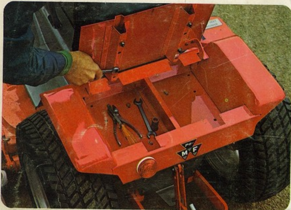
Storage area under seat of MF 10 and MF 12 tractors provides space for carrying tools. Seat is hinged for easy accessibility.
