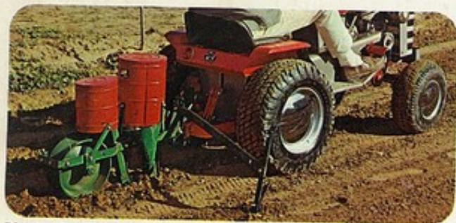
Planter-fertilizer does fast, accurate work in a wide variety of garden crops. Seeding and fertilizing rates can be set. Unit requires MF lift hitch.
