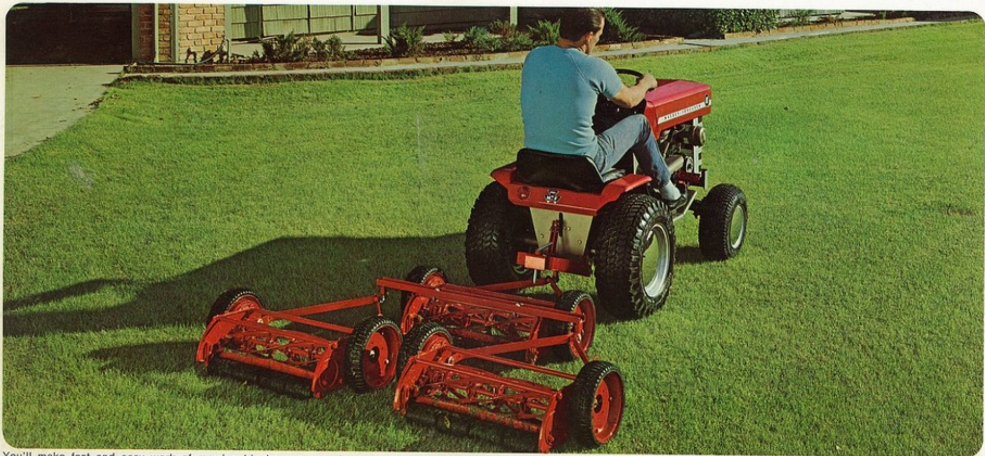
You'll make fast and easy work of mowing big lawn areas with this 3-gang reel mower. You'll be set to cut a 60-inch swath with professional precision and neatness . . . at speeds from 3 to 6 mph. Transport frame and wheels available.
