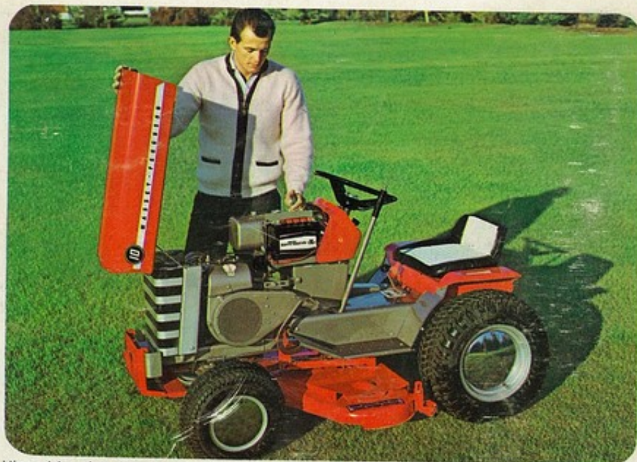
Hinged hood makes it easy to get at engine. With average use you need to grease only three points, twice-a-year!
