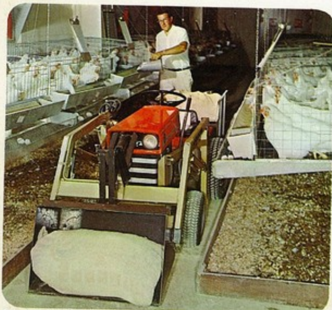
Front-end loader gives the tractors a whole new range of work you can do. Bucket position and lift are controlled hydraulically.
