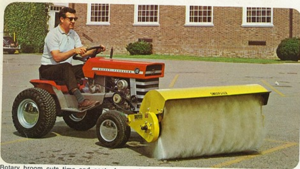
Rotary broom cuts time and cost of sweeping walks, drives, service and parking areas. Airports, too. Long-wearing plastic 48 x 26-inch broom also does good work in light snow. Can be used to remove thatch also.
