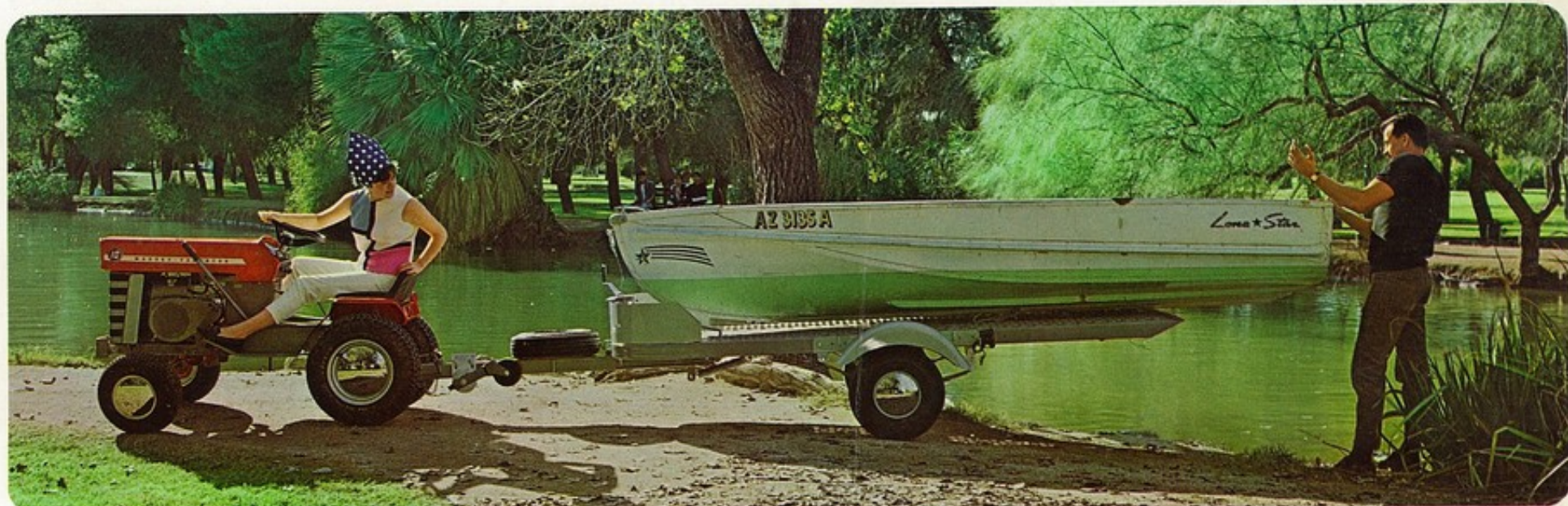
Utility trailer has 46-inch x 111-inch steel platform that tilts to form easy loading ramp. Carrying capacity is 1,000 pounds. Crank winch is optional. Trailer also can be towed by vehicles normally used on highways. You will find many uses for this trailer.
