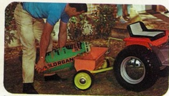
Seed and Fertilizer Spreader has instant flow control start and stop. Also cam-action agitator and calibrated dial. Choice of 30 and 36-inch widths.
