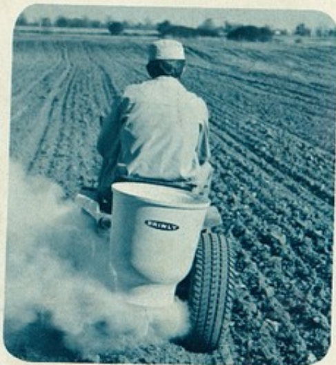
Powr-Caster does top-notch job of spreading everything from salt on icy drives and walks to seed and fertilizer. Spreads pattern to 30 feet wide. Agitator is powered by 12-volt electric motor. Fiberglass hopper holds approximately 100 pounds of fertilizer.
