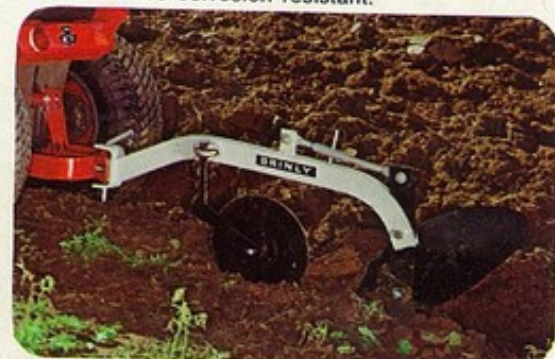
Moldboard plow turns 10-inch furrow. Handy adjustment sets depth to 6 inches. Plow can be lowered and raised by convenient lift lever. Choice of 3 bottoms.
