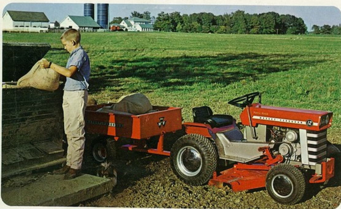
Top chore team! MF 641 dump cart hitched to an MF 10 or MF 12 helps young farmers do things the easy way. They can have some fun doing it, too! Cart has pneumatic tires and all-steel body with removable end gate. Side extensions are available.
