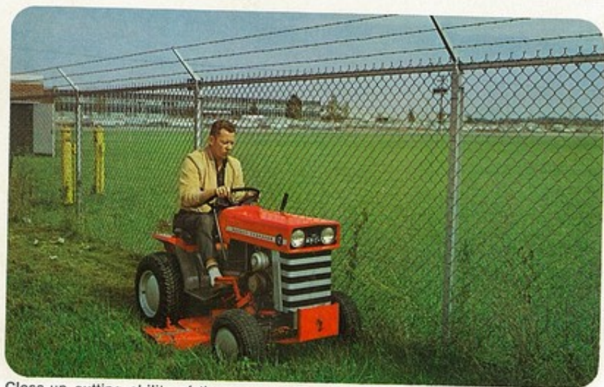
Close-up cutting ability of the rugged MF 610 rotary mower keeps hand trimming to a minimum. Three 15-inch overlapping blades cut heavy growth with ease. Blades remove quickly for sharpening.
