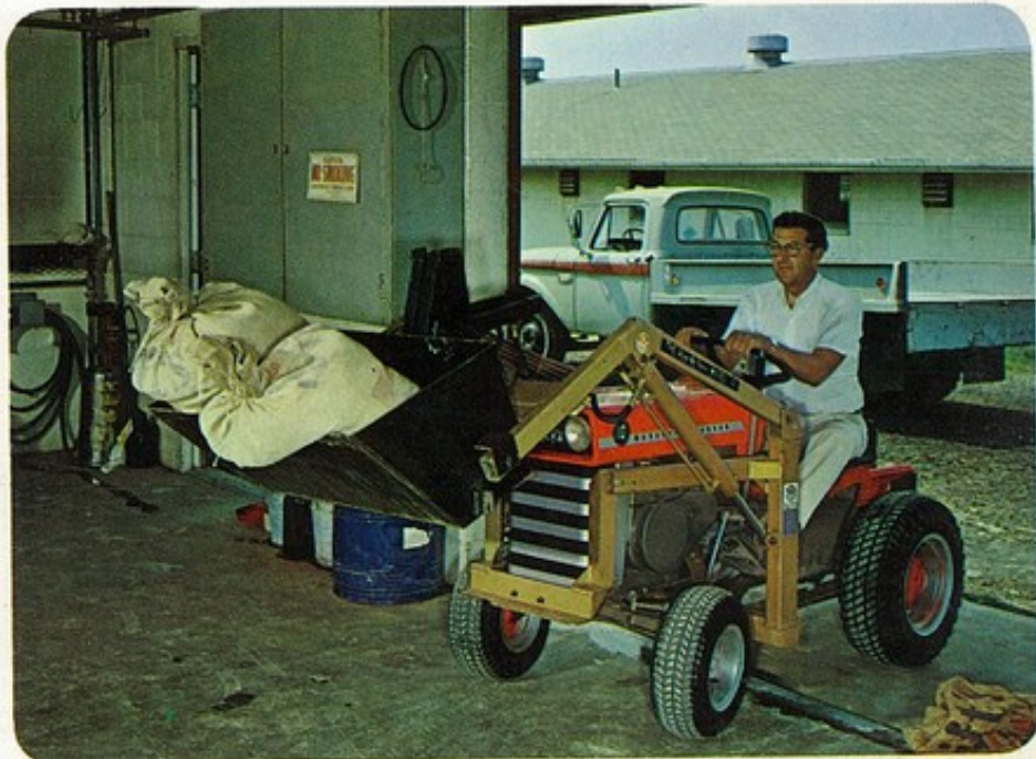
You can lift, load, doze and scrape with this handy hydraulic loader on your MF 10 or MF 12. Loader has 300-pound capacity, 45-inch clearance with bucket in dumped position.
