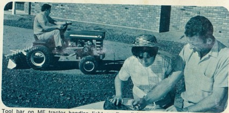
Tool bar on MF tractor handles light grading, finishing, scarifying and backfilling. You'll also find it right for seed bed preparation and cultivating, with optional sweeps.
