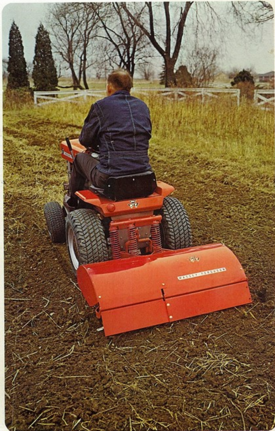
With optional 16-inch extension, the MF 650 rotary cultivating tiller has a full 38-inch working width. Side and rear shields are standard.
