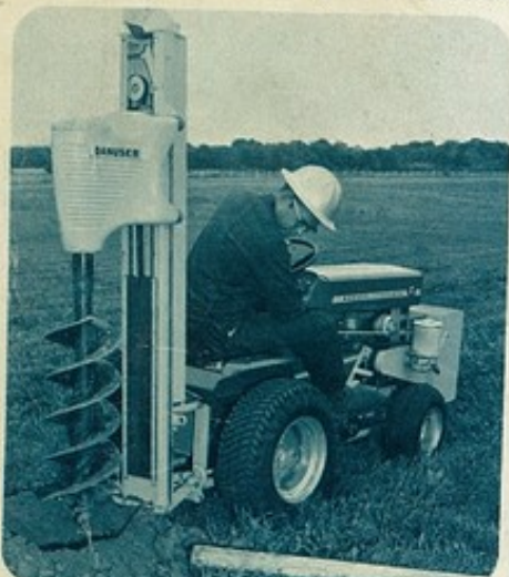
Compact Digger for easy maneuvering in tight places. Digs 30-inches deep with 4, 6, 9, 10, 12 or 14-inch auger. Great for fences, landscapers, nurserymen . . . also parks and cemeteries. Pto driven . . . controlled from tractor seat.
