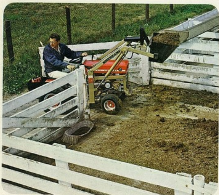
Hydraulic front loader for the tractors takes the back-work out of cleaning and loading manure and materials in close quarters. You can get in and out with an MF 10 or MF 12. Choice of three buckets.
