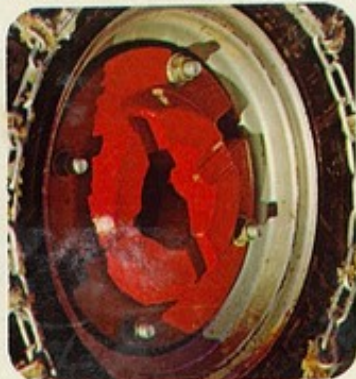
Wheel weights are available for both MF tractors. They bolt on to rear wheels, provide added traction for hard pulling loads.
