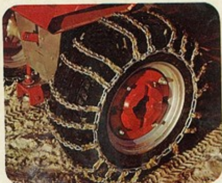
Tire chains will equip you to make better use of your MF tractor's power in snow and other work where extra traction is needed.
