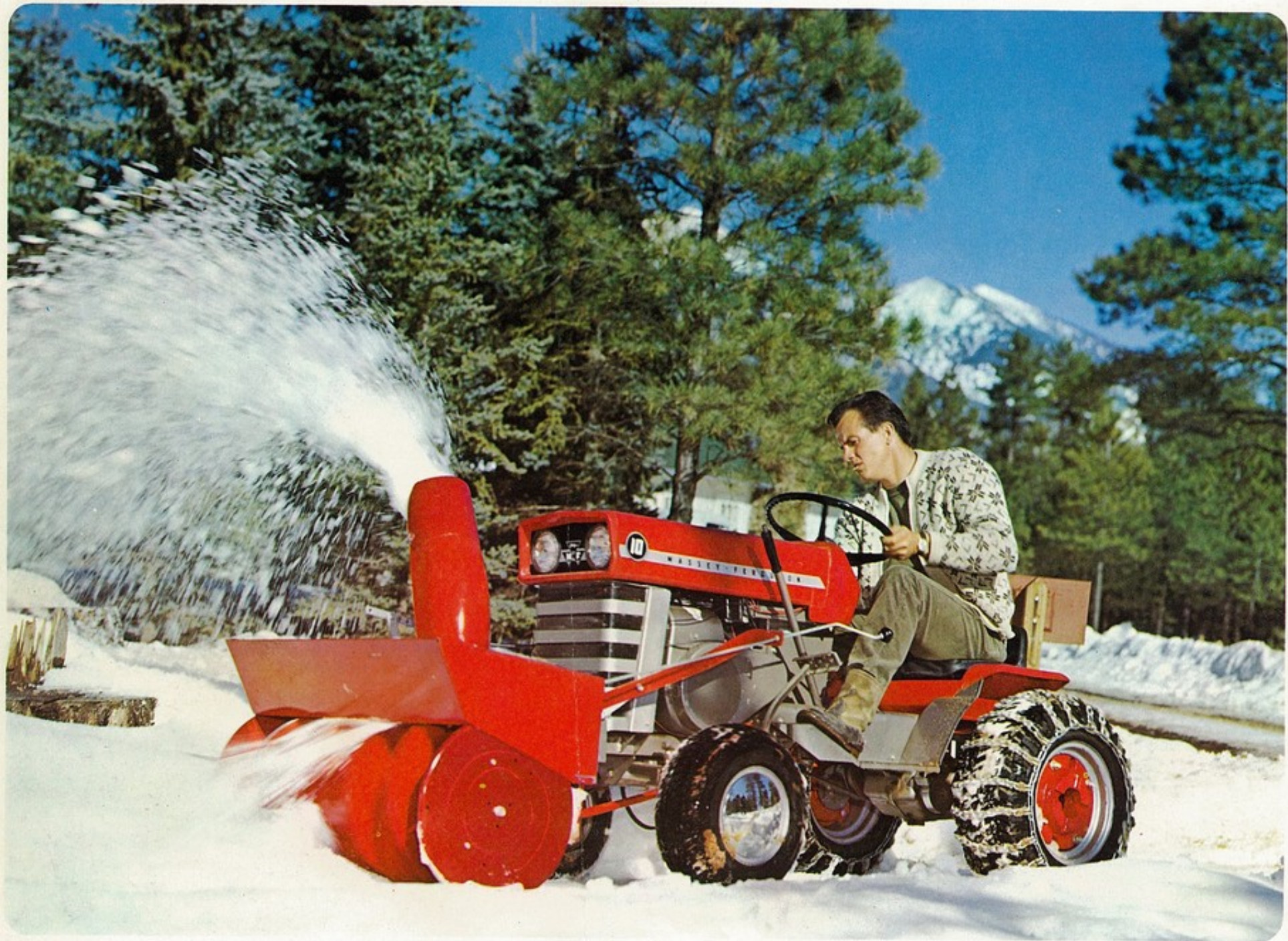
You can shoot 36-inch snow swath to 20 feet or more with this MF 620 Snow Thrower. Handy control crank rotates 270° to throw snow 135° to right or left, as you like.
