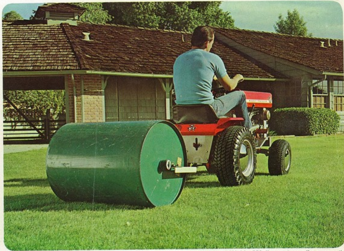
Lawn roller helps you firm new seed beds, also smooth existing lawns. Holds 550 lbs. water, rolls a smooth 32-inch width. Scraper blade provides self-cleaning action to keep rolling surface clear for best work. Easy draw bar attachment puts you on the job in a hurry.
