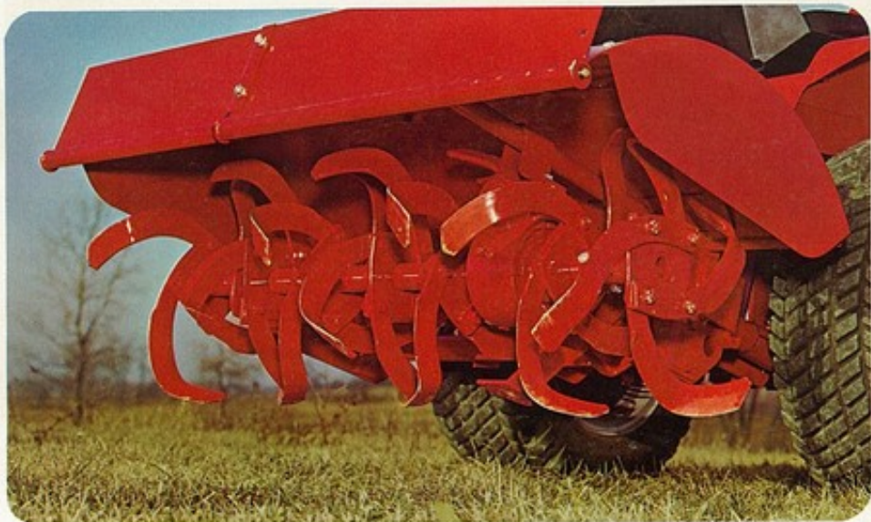
MF cultivating tiller mounts in-close on tractor lift hitch. Lift lever lets you raise, lower unit on-the-go for fast turn-arounds at row ends.
