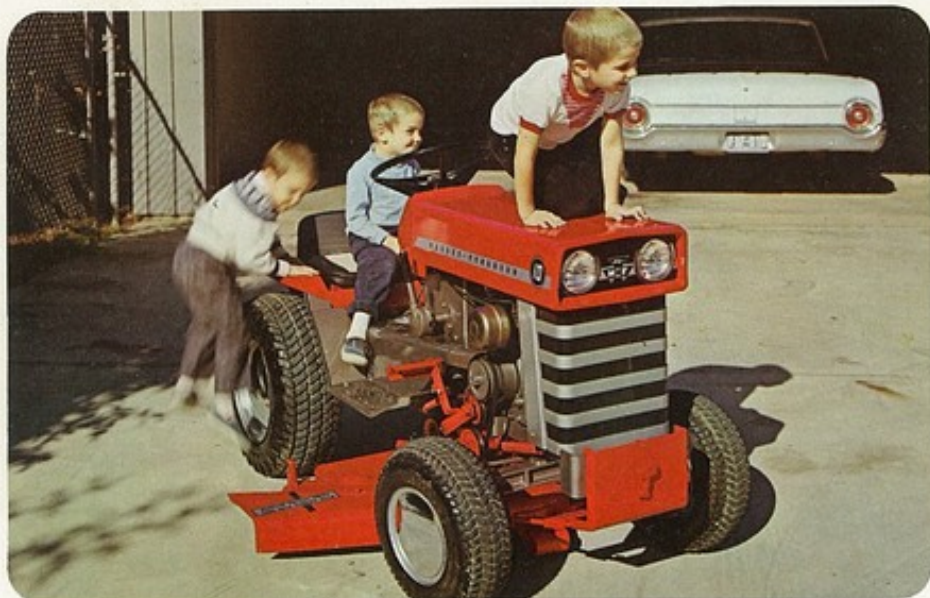
Let 'em play! You can pocket the ignition key. And for added safety, the traction belt is declutched when the parking brake is engaged. Drive shields and fenders are standard on MF tractors for added protection.
