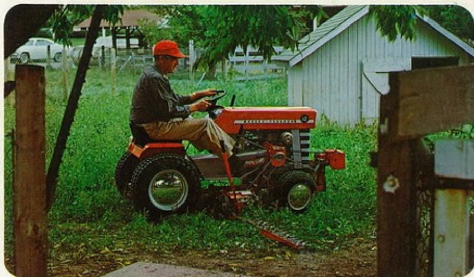
Sickle bar mower on MF 10 or MF 12 gives you a compact unit that lets you mow areas too small for big rigs. Cutter bar also locks at near vertical angle for trimming sides of hedges. Cutter bar cuts full 4-foot swath.
