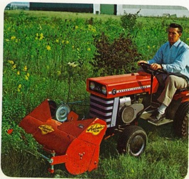
Flail mower puts the MF pto power to good use if you have heavy-duty mowing. Rugged chopping action shreds grass, mulches leaves. Mower is 36 inches wide.
