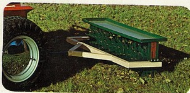
Spike aerator has weight pan and reversible teeth for smooth or rough spiking. Covers 32-inch swath. Axle is roller-bearing mounted for easy pulling and less wear.
