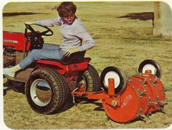
Lawn aerator breaks up thatch for the stimulation good grass needs. Cast steel tubes make 8 x 8-inch hole pattern in 2-foot swath. Tank can be filled with water.
