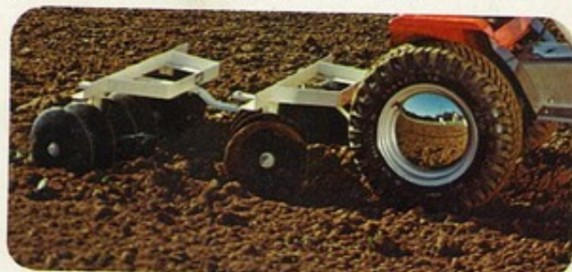
Disc-harrow is available with single or double row of discs, adjusts to 10°, 15° or 20° angles for widths 29 inches to 39 inches. MF lift hitch required.
