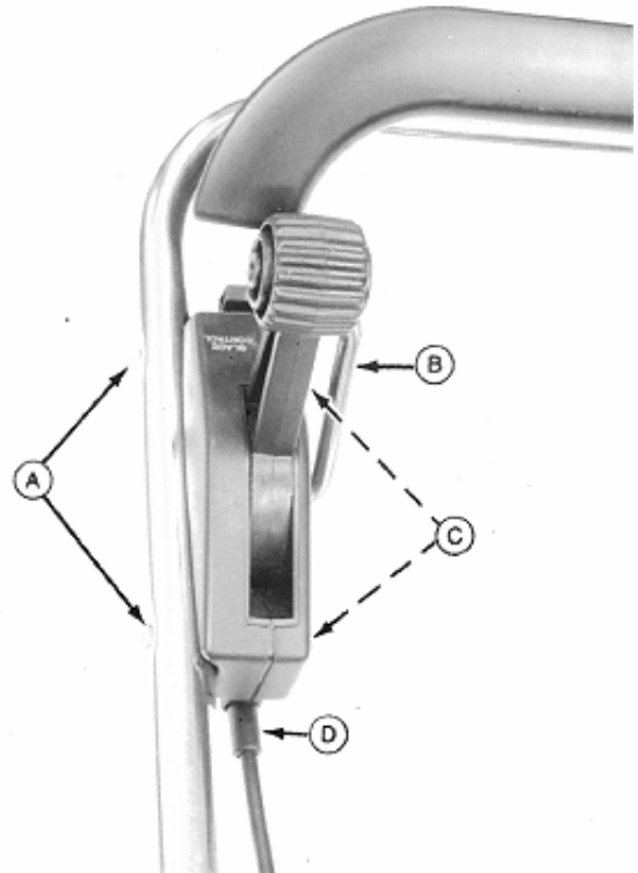
A—Mounting Cap Screws B—Safety Bail C—Lock Nuts D—Control Cable
