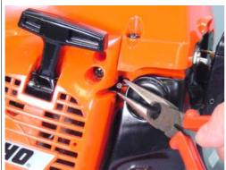
1. Turn the L and H mixture needles out anticlockwise to rich side stop, and meet limiter caps tabs (A) with locating slots (B).
