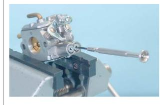
8. Turn L and H mixture needles clockwise until lightly seated using 1.5mm blade screw driver, and then turn both needles anticlockwise for following turns.
