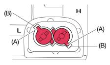
2. Screw 2.5 mm wood screw in the center of the L limiter cap.
