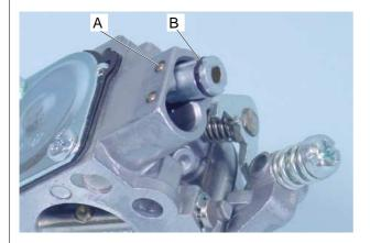
7. Temporally insert new limiter caps on both L and H mixture needle by aligning groove on limiter cap (B) to locating pin (A) on extension housing. Make it sure that limiter cap face is leveled with extension housing top. Do not press limiter cap deeper at this moment.
