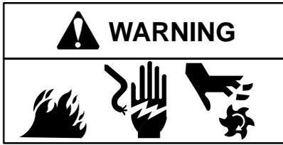
If you perform any maintenance on the engine, first disconnect the spark plug wire from the spark plug, and disconnect the battery at the negative terminal (electric starter engines only) to prevent unintentional sparking. Unintentional sparking can result in fire or electric shock. Unintentional start-up can result in entanglement, traumatic amputation or laceration. Use only correct tools.
