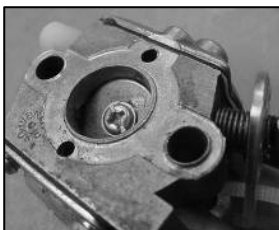
Worn Mounting Surface
