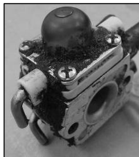
Fuel Leak Indicated by Dirt Build-up
