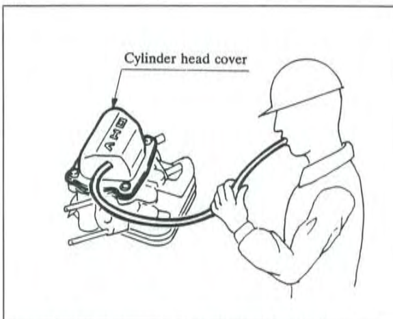
Checking breather valve (Simplified method)
