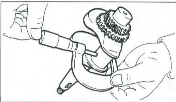
Measuring crank pin outer diameter
