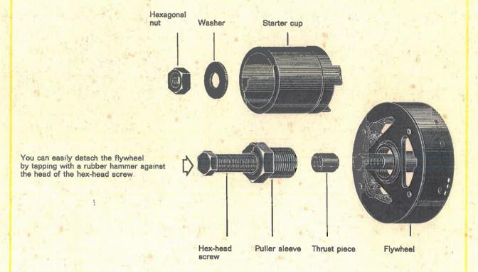
Place thrust piece on crankshaft. Unscrew hex-head screw until puller sleeve can be slid over the thrust piece, and screwed into the flywheel until it reaches the limit stop. Screw in hex-head screw with a 17 mm (67 in.) socket wrench with a sufficiently long handle until flywheel snaps off. The stator plate is attached to the crankcase by two cylindrical screws. Remove ground wire from toggle switch.
