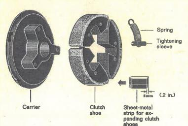
The clutch consists of 3 clutch shoes, 3 clutch springs, 6 tightening sleeves and the clutch carrier.
