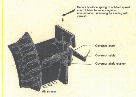
For protecting governor shaft, governor shaft retainer and coils of hook-on spring against ice and resin apply a few drops of kerosene on all parts.
