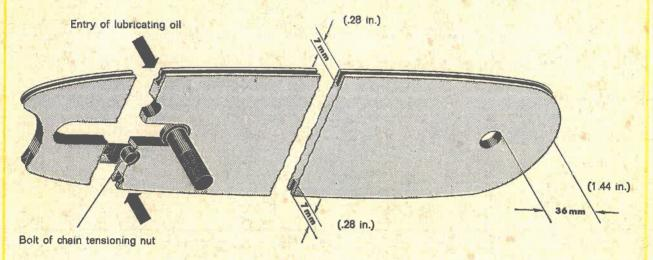
If bar wear exceeds the limit of 36 mm (1.44 in.) and 7 mm (.28 in.) respectively the bar must be reconditioned.
