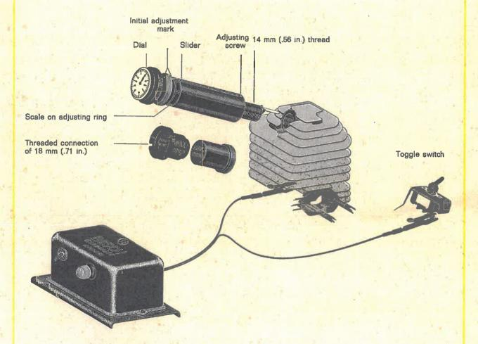
Before installing or removing timing gauge from spark plug hole, make it a rule to put adjusting ring and slider to -0- position.
