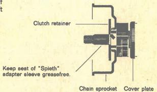
Tighten hexagonal nut with torque wrench set to 4.5 to 5 mkg (32—36 ft. lbs.). When tightening nut the crankthrow should not knock against the crankshaft stop, but rest on it.
