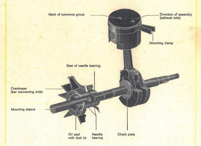
For protecting the oil seals against damage, use the mounting sleeve when mounting the crankshaft. Make sure, that the sealing surfaces at the crankcase half and the gaskets are not damaged. Don't use cementing material, otherwise the crankcase may be contaminated.
