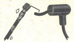
When attaching a new ignition wire to the stator plate, don't forget to slide the guard socket over the connection. Apply ignition grease to guard socket and wire end. Thread other wire end through grommet and crankcase hole to carburetor side.
