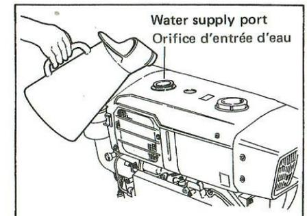
(A) Do not use hard water nor water containing foreign matter or mud. The hard water such as well water difficult to soap will decrease cooling efficiency in the cylinder because of its deposit.
